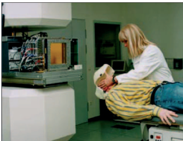
▲ Fig. 5: The GSI horizontal beam has been used to treat mainly intracranial and head and neck tumours. The two white boxes, placed above and below the patient, contain the detectors for the on-line PET measurement of the stopping particles.
